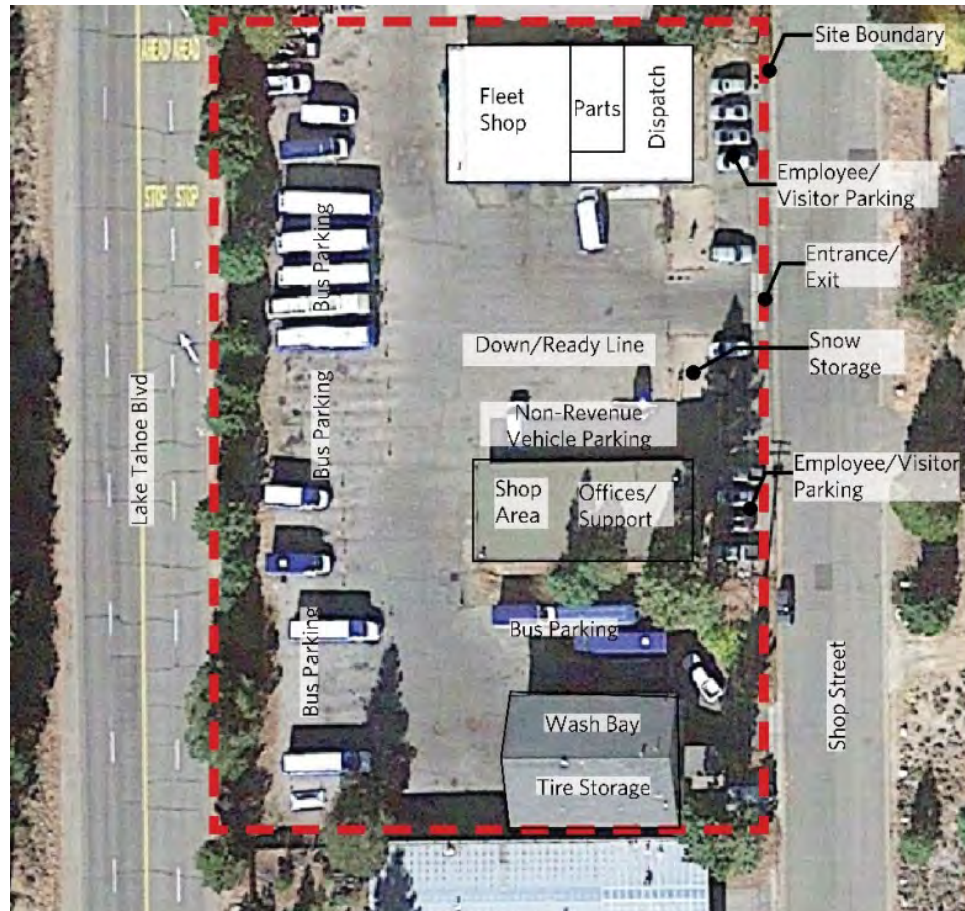
Figure 3-5: TTD Operations and Maintenance Facility (Source: TTD Bus Ops., Maint., and Admin. Facility Master Plan)
