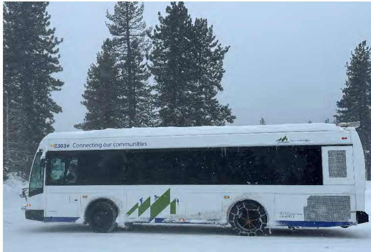
Figure 6-2 - Chained Bus During Winter
