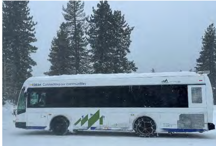
Figure 6-2 - Chained Bus During Winter
